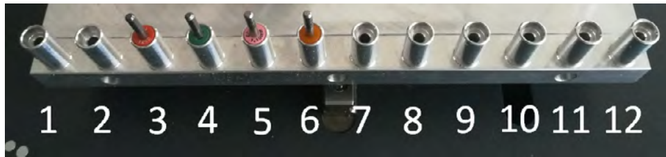
Figure 22 – real tool changer bar with correctly inserted tools
