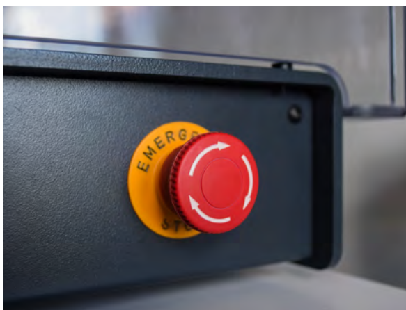
Figure 3 – safety and power switch and its connection
