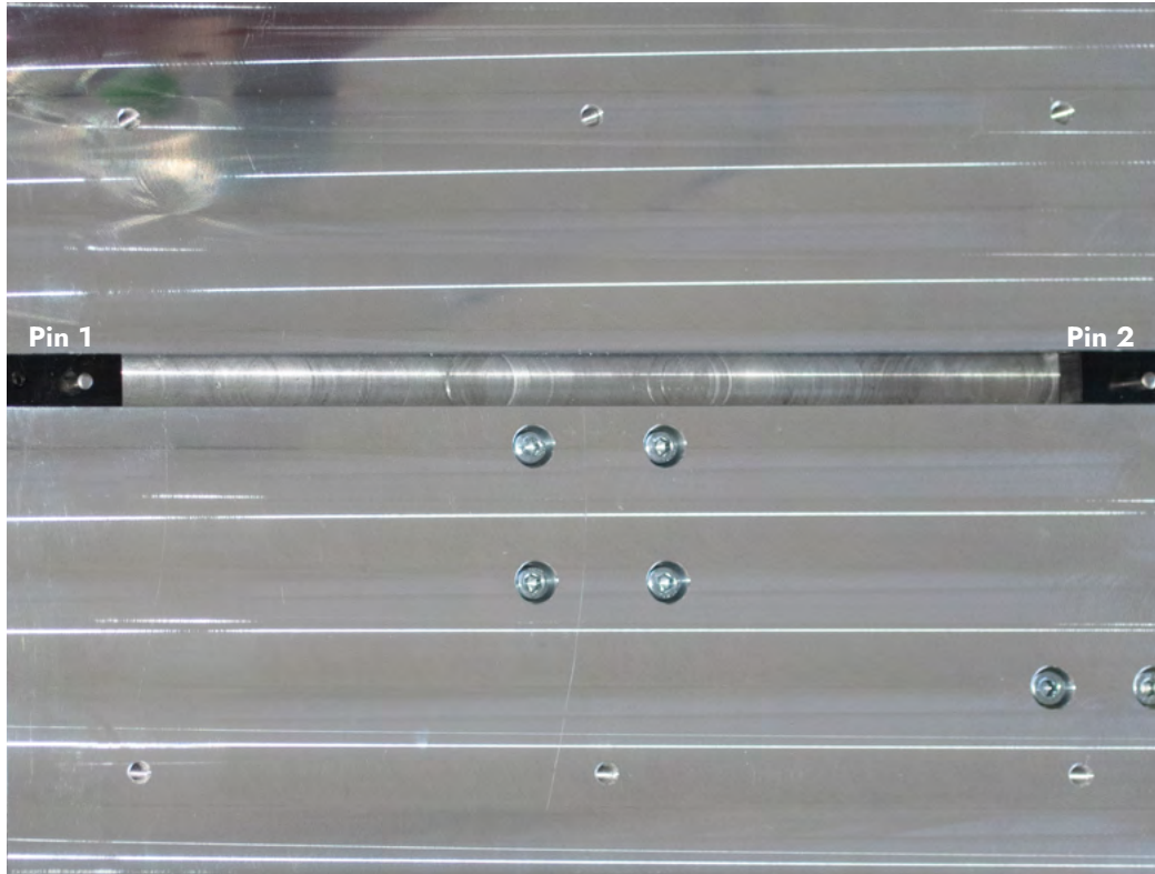
Figure 10 – machine table with mounting pins and central T-groove
